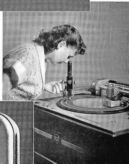
FIG. 6. The RCA 73-B Professional Recorder may be used to cut grooves at "three" speeds (78, 33 1/3 and 45).
