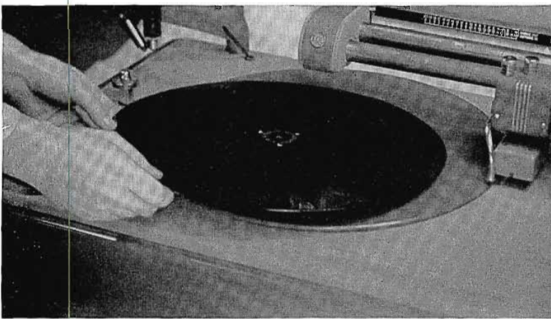
ANY TYPE BLANK may be used with the single driving pin provided. Here, recording blank is placed in position.
