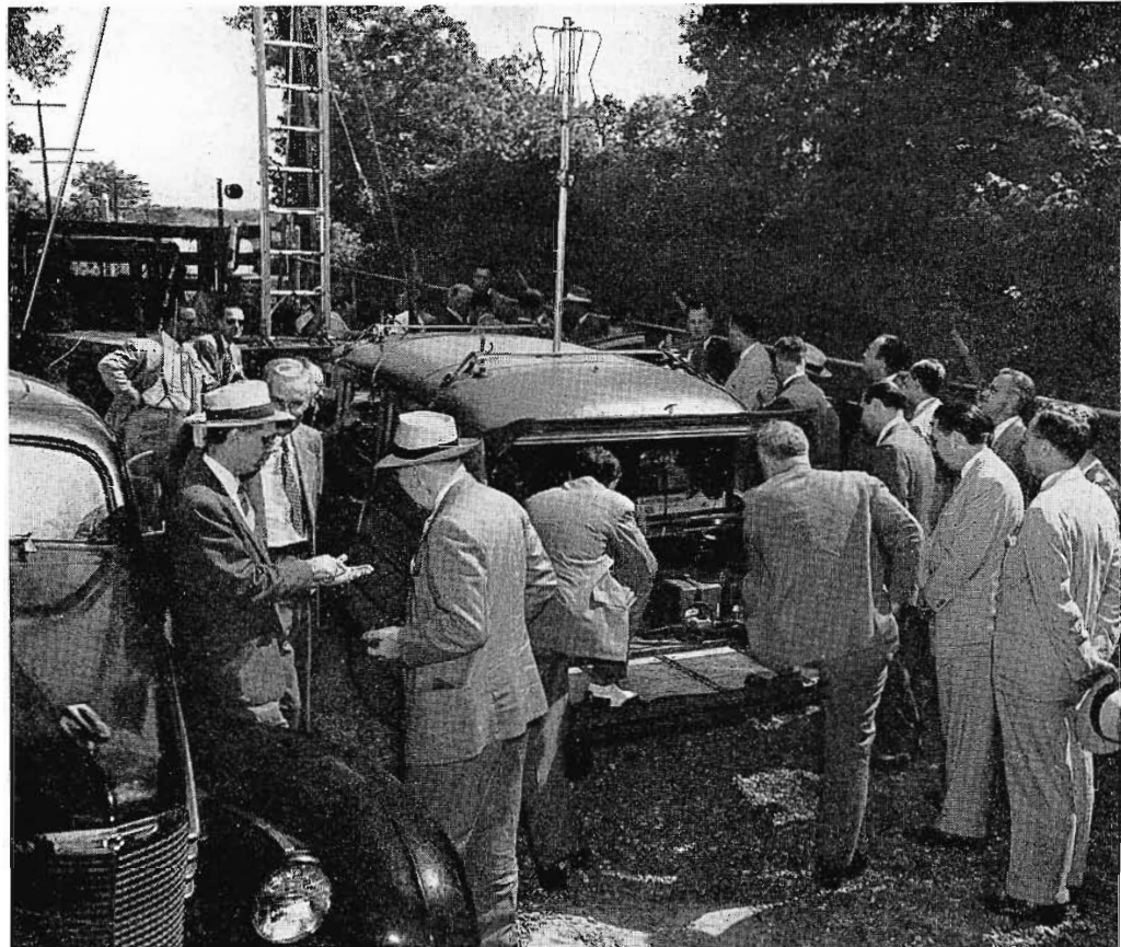
Visiting engineers and attorneys inspect the "UHF Caravan" used by NBC in making field surveys of the UHF TV signal. Two vehicles are used. Station wagon in foreground contains a modified RCA Type WX-1A UHF Field Intensity Meter, recorders, altimeter, telephone communications equipment and a Super-Turnstile type receiving antenna mounted at a 10-foot height. Correlations between this antenna and one mounted on the truck at a 30-foot height (on the ladder in the foreground) are made from the recordings on each antenna. Photo below is a view inside station wagon. Receiver at left has built-in converter which feeds the 21 mc receiver i-f stages.
